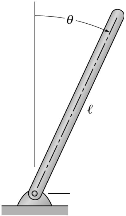
Inverted compound pendulum with an unstable static equilibrium position about  $\theta = 0$ .
