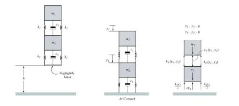
At the left is an assembly that is released from a height h = 2ftabove the ground. In the middle, the assembly has just contacted the ground. The subsequent positions of  $m_1$  and  $m_2$  are defined, respectively, by  $y_1$  and  $y_2$ . At the time of contact,  $y_1(0) = y_2(0) = 0$ , and  $\dot{y}_1(0) = \dot{y}_2(0) = v_0 = \sqrt{2gh} = \sqrt{2 \times 32.2 \times 2} = 11.35 ft/sec$ ...
