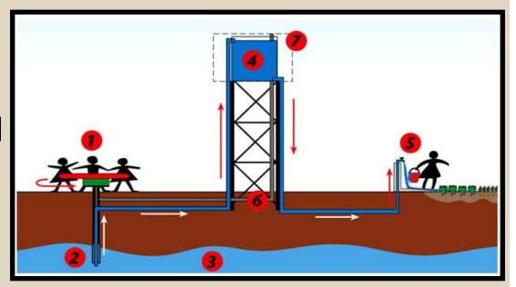
Capabilities: 1,400 liters of water per hour at 16 rpm from a depth of 40 meters
