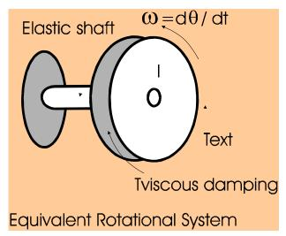
external moment or torque, and  $\theta(t)$  is the angular displacement of the rotational system.
