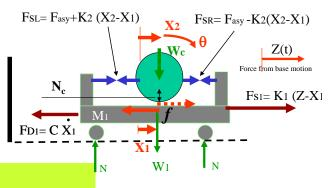
$$\underline{Kinetic\ energy} = T = T_{\text{trailer\ translation}} + T_{\text{Tcylinder\ - translation}} + T_{\text{cylinder\ - translation}}$$
