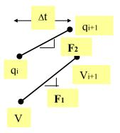
$$\frac{V_{i+1} \sim V_i + \Delta t \, f_{1_i}, \quad f_{1_i} = F_1(q_i, V_i, t_i),}{q_{i+1} \sim q_i + \Delta t \, f_{2_i}, \quad f_{2_i} = F_2(q_i, V_i, t_i)} \quad \text{for } i = 1, 2 \dots \dots \quad (A.7)$$
