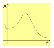
$$F_{K}(t) = -F_{o}A\sin(\Omega t - \varphi) \approx -F_{o}1\sin(\Omega t - 0) \approx -F(t)$$
