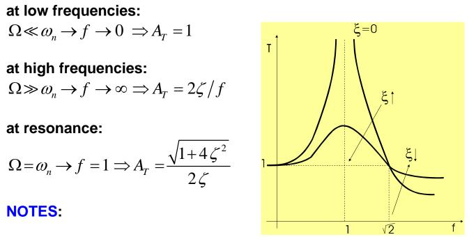
At low frequencies,  $f < \sqrt{2}$ , the transmitted force (to base) is larger than external force, i.e. T > 1
