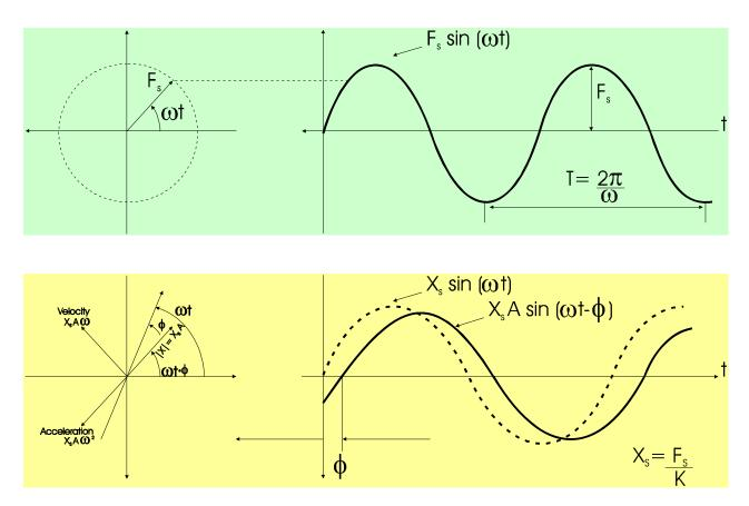
Note that the **velocity**  $\dot{X}$  leads by 90° the displacement X(t), and the **acceleration**  $\ddot{X}$  leads by 180° the displacement X(t).
