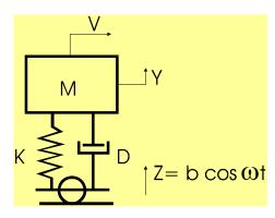
The wavelength is equal to  $\lambda = v T$ , with T as the period of motion. And the frequency ( $\omega$ ) of the forced motion is:
