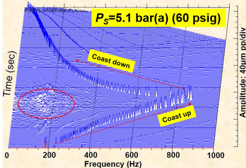
**Procedure:** Rotor accelerates the rotor to 55 krpm (910 Hz). Motor is shut off and rotor coasts down to rest.
