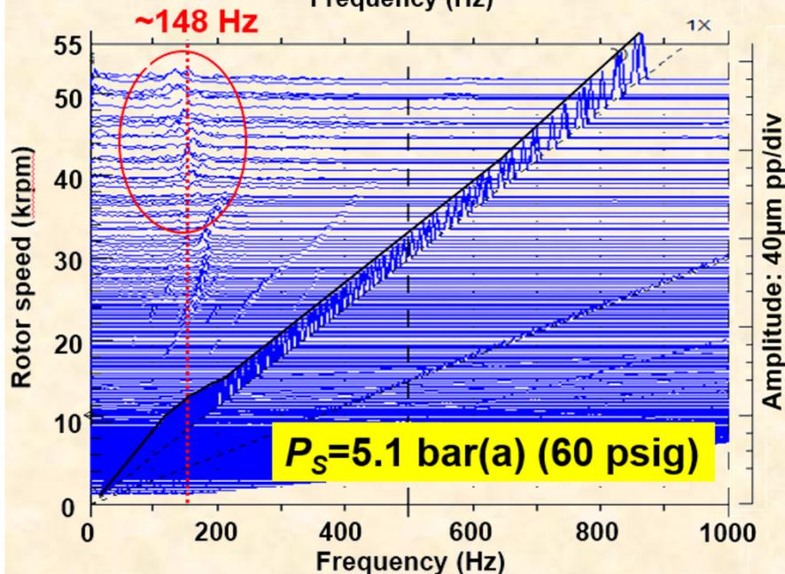
**Findings:** The rotor response is mainly synchronous (1X). Incipient subsynchronous motion appear at speed above 2 x natural frequency. Whirl then locks at the natural frequency. The rotor-bearing system does not show a self-excited whirl instability.
