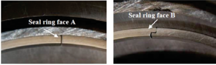
Fig. 24. Proper installation of piston ring in bearing cartridge: face A towards ambient [14].
