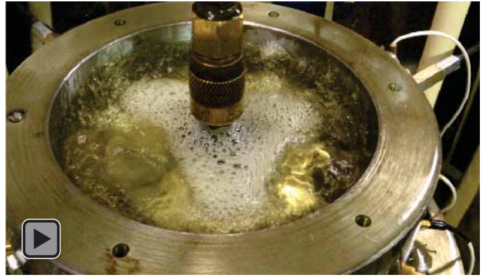
Fig 8. Video depicting outlet foamy lubricant in an open ends SFDs. http://youtu.be/8wQ1TnGTmyE
