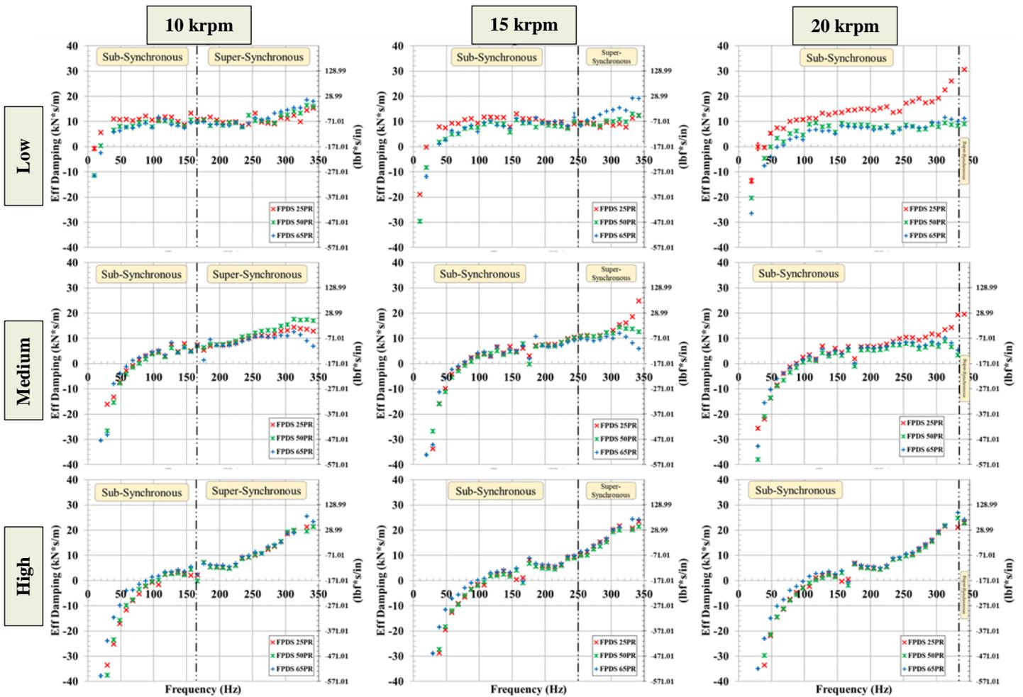
Figure 12 FPDS effective damping coefficient ( $C_{eff}$ ) versus excitation frequency for tests at three pressure ratios (25%, 50%, 65%), three inlet pre-swirls (low, medium, high), and three rotor speeds (10, 15, 20 krpm).
