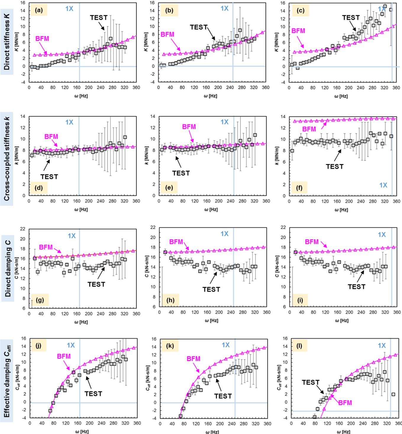
Figure 22 FPDS: test and BFM predicted force coefficients ( $K$ ,  $k$ ,  $C$ ,  $C_{eff}$ ) vs. frequency ( $\omega$ ) for  $P_{in} = 70$  bar,  $PR = 0.5$ . Shaft speeds: 10, 15 and 20 krpm ( $\frac{1}{2}QD = 60$  to 120 m/s), medium inlet pre-swirl condition.
