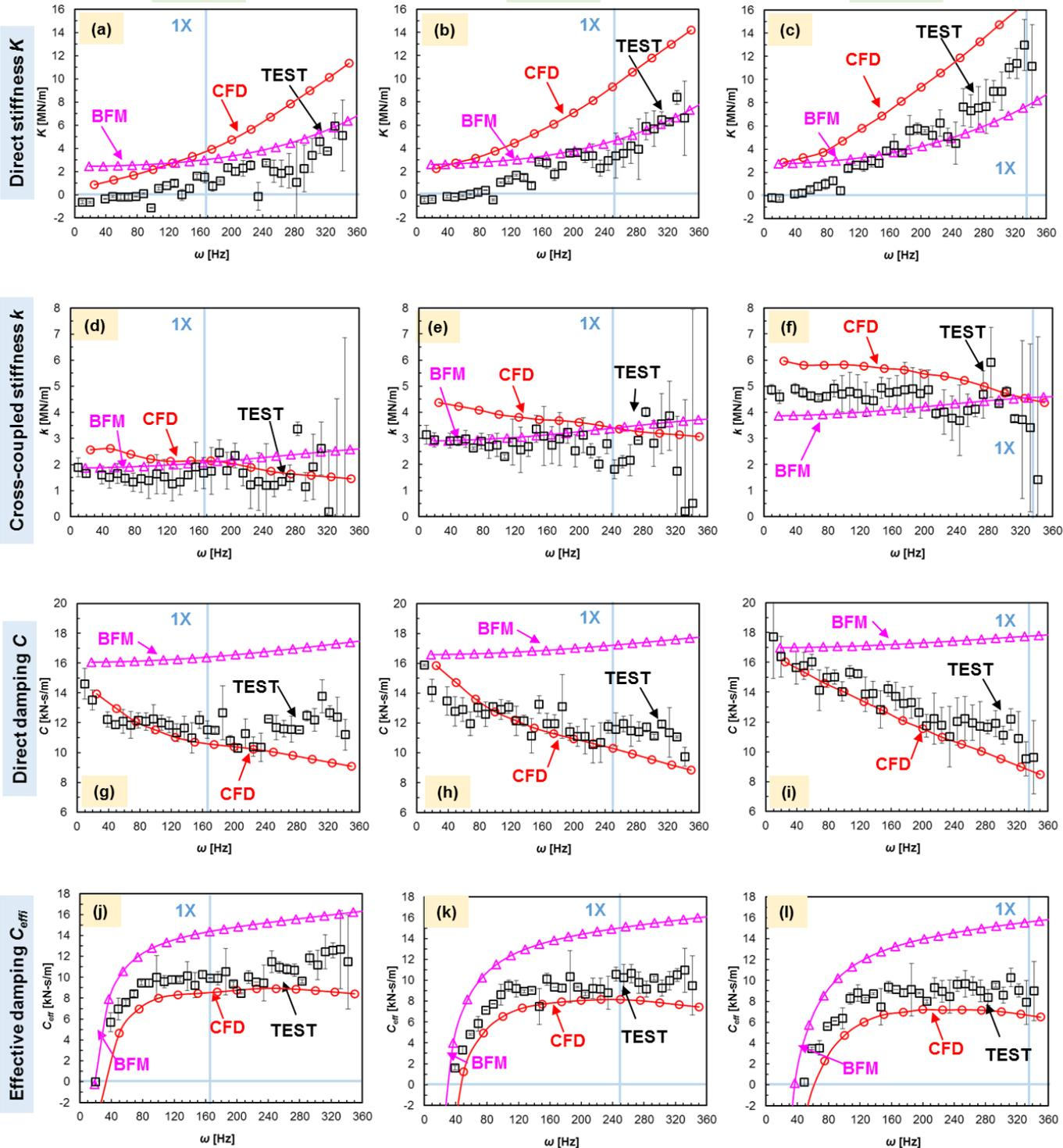
Figure 19 FPDS: test, CFD and BFM predicted force coefficients ( $K$ ,  $k$ ,  $C$ ,  $C_{eff}$ ) vs. frequency ( $\omega$ ) for  $P_{in} = 70$  bar,  $PR = 0.5$ . Shaft speeds: 10, 15 and 20 krpm ( $\frac{1}{2}QD = 60$  to 120 m/s), zero inlet pre-swirl conditions.
