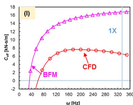
Figure 20 FPDS: test, CFD and BFM predicted force coefficients ( $K$ ,  $k$ ,  $C$ ,  $C_{eff}$ ) vs. frequency ( $\omega$ ) for  $P_{in} = 70$  bar,  $PR = 0.25$ . Shaft speeds: 10, 15 and 20 krpm ( $\frac{1}{2}\Omega D = 60$  to  $120$  m/s), zero inlet pre-swirl conditions.
