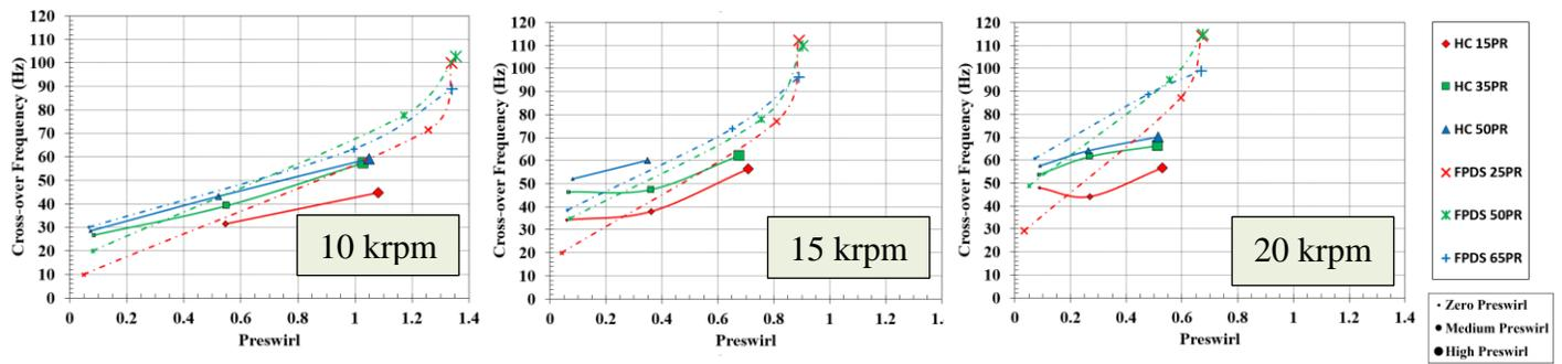
**Figure 16** Cross-over frequency versus ( $\omega_{co}$ ) inlet pre-swirl ratio ( $\alpha$ ) for FPDS and honeycomb seal (HC) [5]. Multiple pressure ratios  $PR = 15\% - 65\%$  and three rotor speeds (10, 15, 20 krpm). Inlet pre-swirl obtained with low, medium and high pre-swirl rings.
