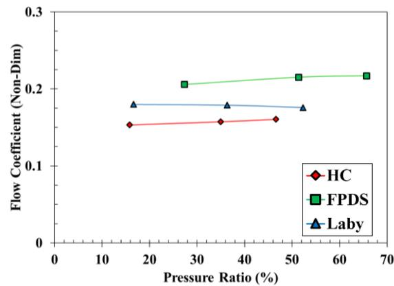
**Figure 17** Flow coefficient ( $\bar{\phi}$ ) vs. pressure ratio for honeycomb seal (HC) [21], fully partitioned pocket damper seal (FPDS), and labyrinth seal (LS) [34]. Average from operation at three shaft speeds (10, 15, 20 krpm). Seals with medium inlet-swirl ring.
