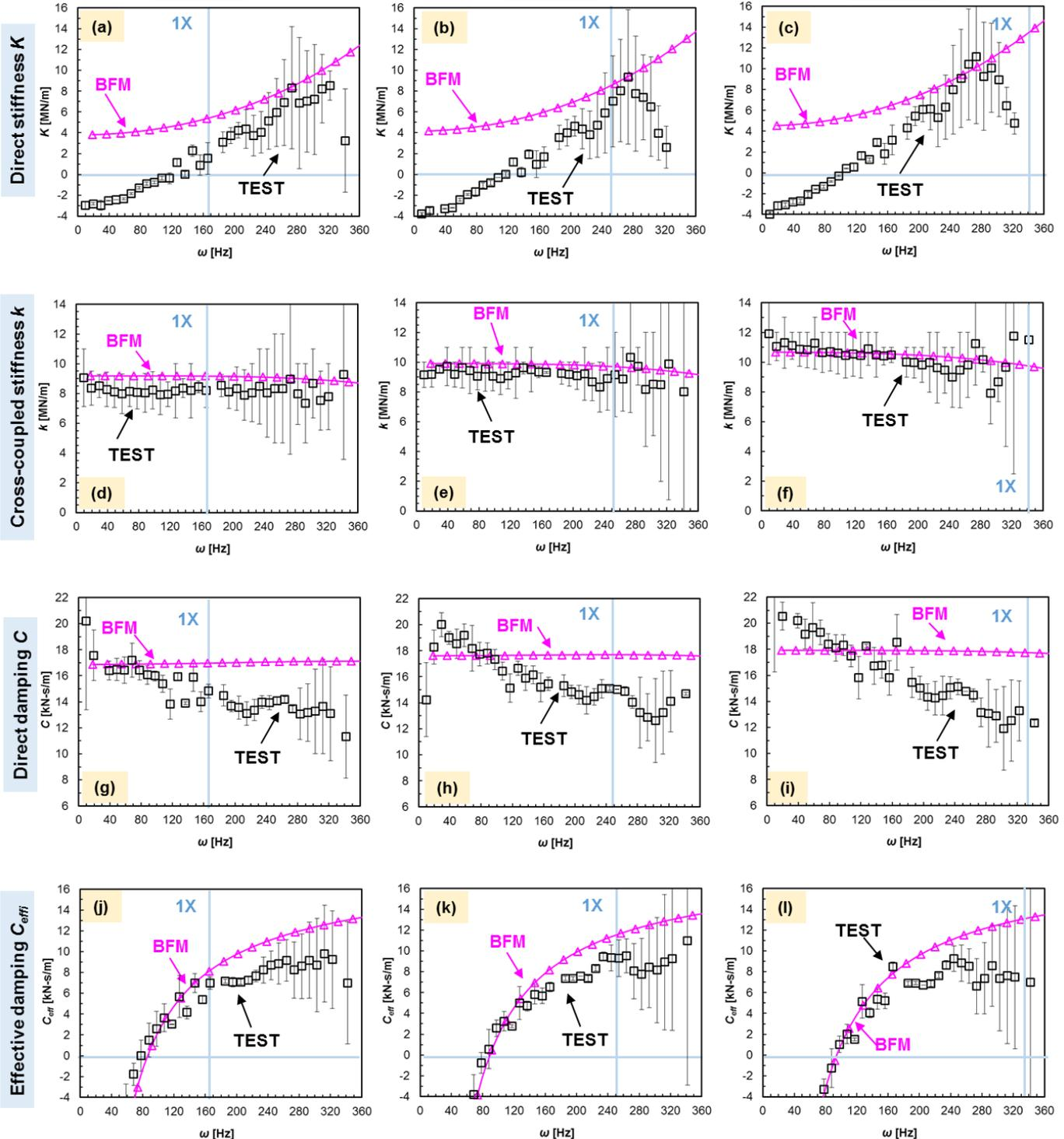
Figure 23 FPDS: test and BFM predicted force coefficients ( $K$ ,  $k$ ,  $C$ ,  $C_{eff}$ ) vs. frequency ( $\omega$ ) for  $P_{in} = 70$  bar,  $PR = 0.25$ . Shaft speeds: 10, 15 and 20 krpm ( $\frac{1}{2}\Omega D = 60$  to  $120$  m/s), medium inlet pre-swirl condition.
