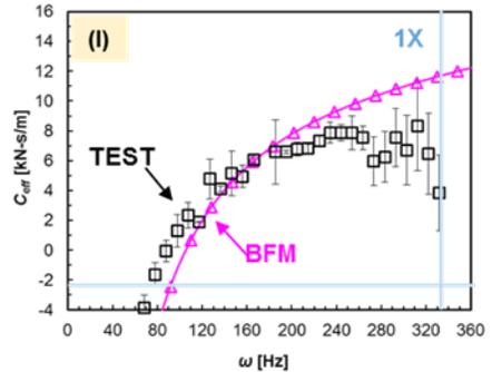
Figure 21 FPDS: test and BFM predicted force coefficients ( $K$ ,  $k$ ,  $C$ ,  $C_{eff}$ ) vs. frequency ( $\omega$ ) for  $P_{in} = 70$  bar,  $PR = 0.65$ . Shaft speeds: 10, 15 and 20 krpm ( $\frac{1}{2}\Omega D = 60$  to 120 m/s), medium inlet pre-swirl condition.
