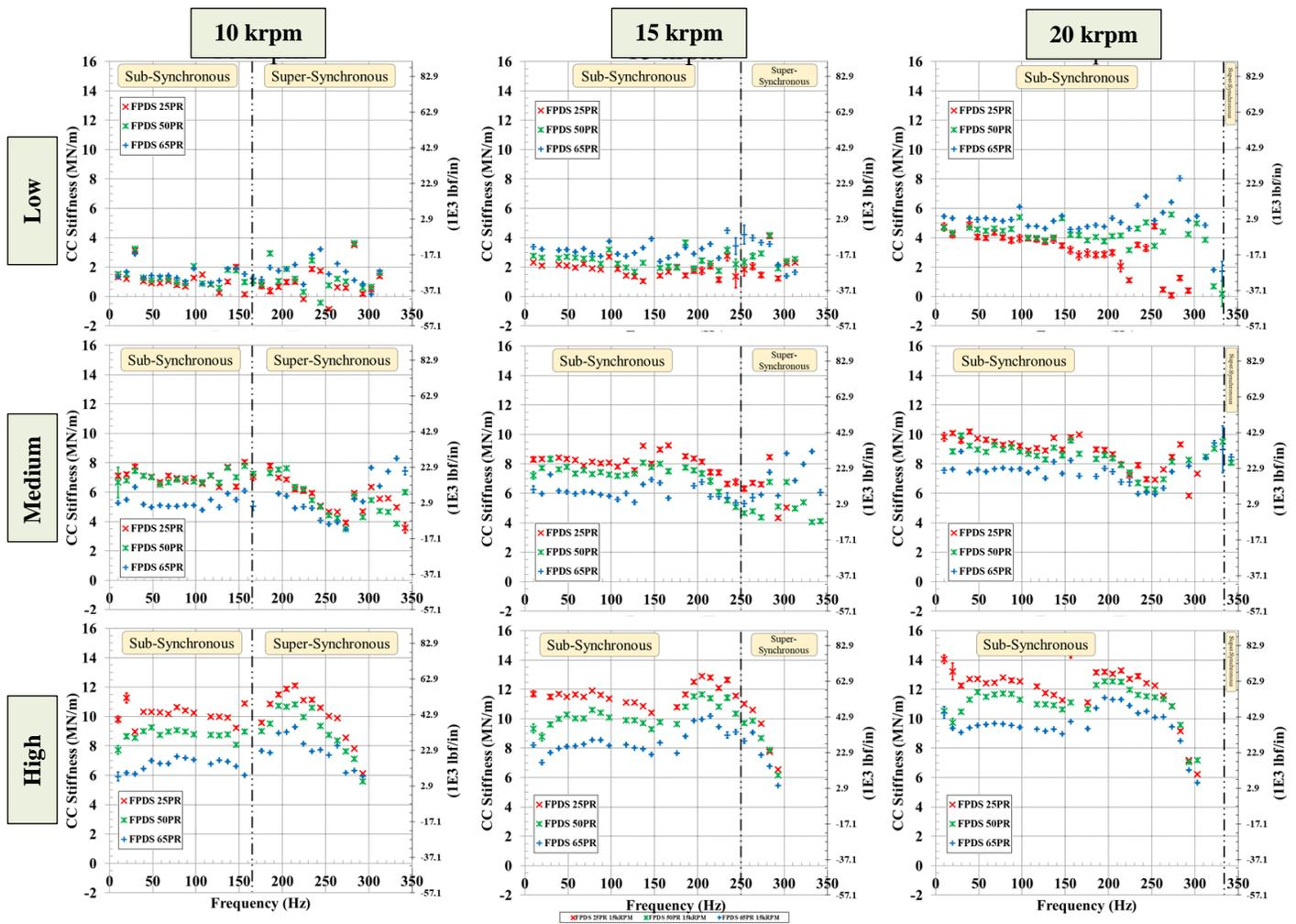
**Figure 10** FPDS cross-coupled stiffness coefficient ( $k$ ) versus excitation frequency for tests at three pressure ratios (25%, 50%, 65%), three inlet pre-swirls (low, medium, high), and three rotor speeds (10, 15, 20 krpm).
