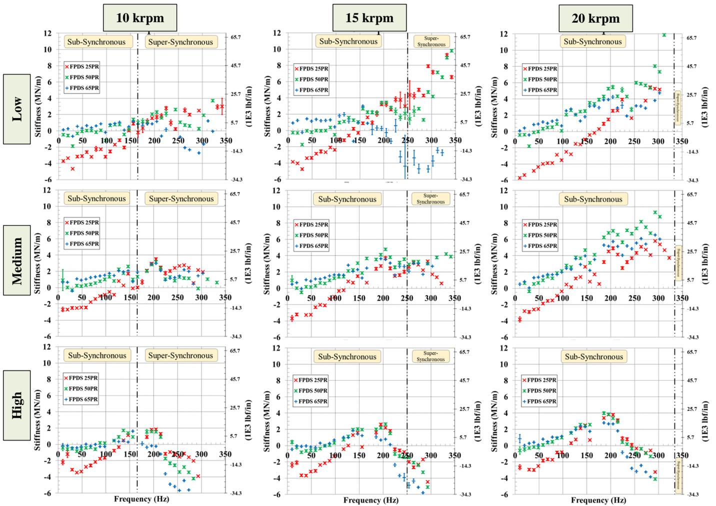
Figure 9 FPDS direct stiffness coefficient ( $K$ ) versus excitation frequency for tests at three pressure ratios (25%, 50%, 65%), three inlet pre-swirls (low, medium, high), and three rotor speeds (10, 15, 20 krpm).
