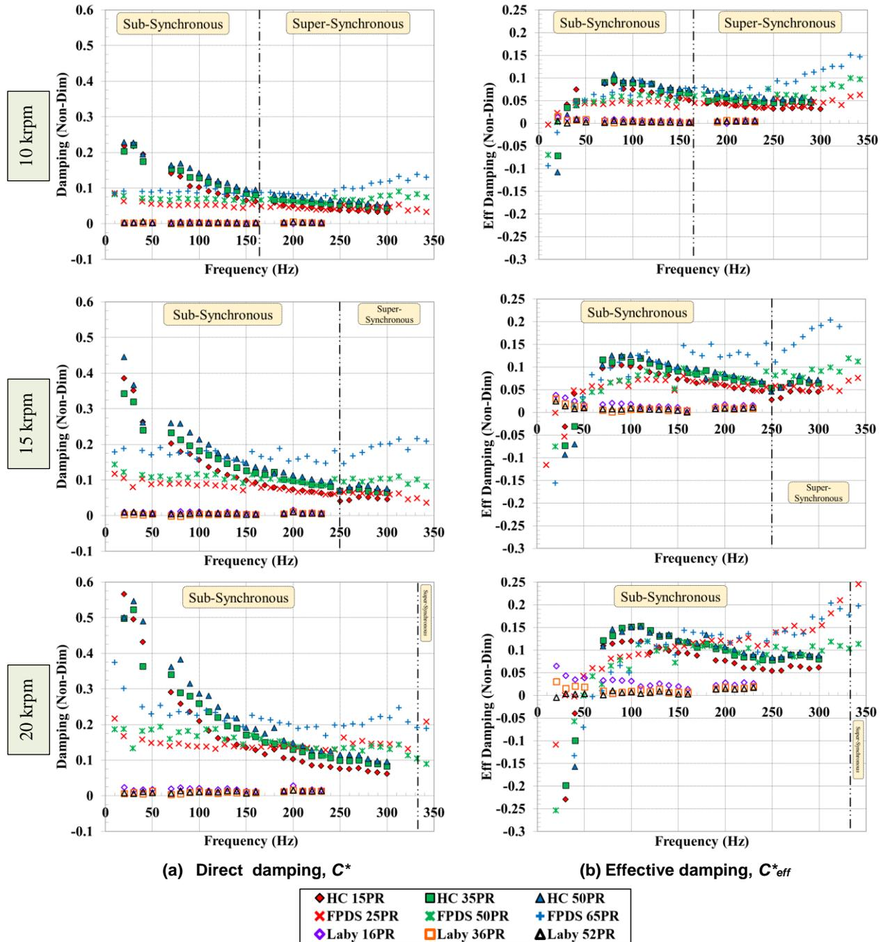
**Figure 15 (Normalized) Direct damping ( $C^*$ ) and effective damping ( $C_{eff}^*$ ) coefficients versus frequency for pocket damper seal (FPDS), honeycomb seal (HC), and labyrinth seal (LS). Multiple pressure ratios  $PR = 15\% - 65\%$ , three rotor speeds (10, 15, 20 krpm), and a low inlet pre-swirl condition ( $\alpha < 0.1$ ) for the three seals.**
