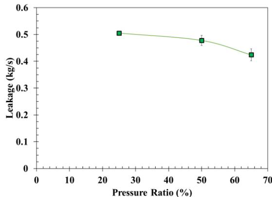
Figure 13 FPDS leakage versus pressure ratio ( $PR$ ). Mean value from tests conducted at three shaft speeds (10, 15, 20 krpm). Seal installed with the medium pre-swirl ring and the high pre-swirl ring.
