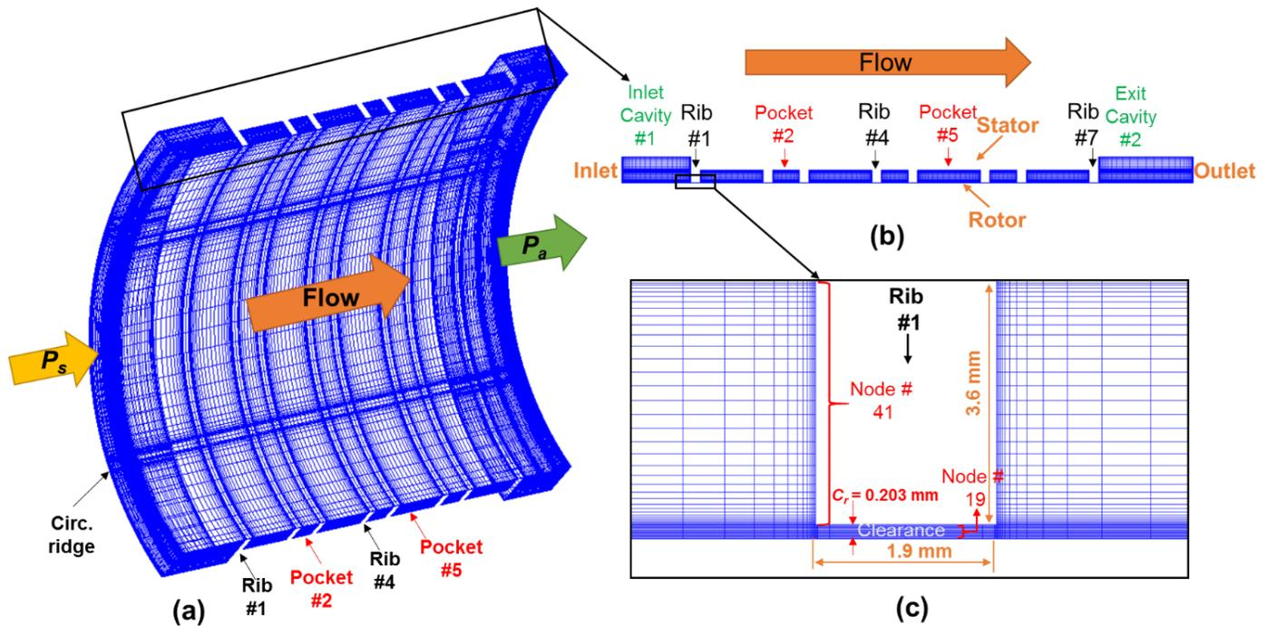
Figure 7 Three-dimensional mesh for an eight-rib fully partitioned damper seal. (a)  $\frac{1}{4}$  cut ( $90^\circ$ ) of three-dimensional mesh; (b) a cross-section view of the mesh; and (c) mesh details around the first rib (#1) ( $L/D = 0.75$ , clearance = 0.203 mm).
