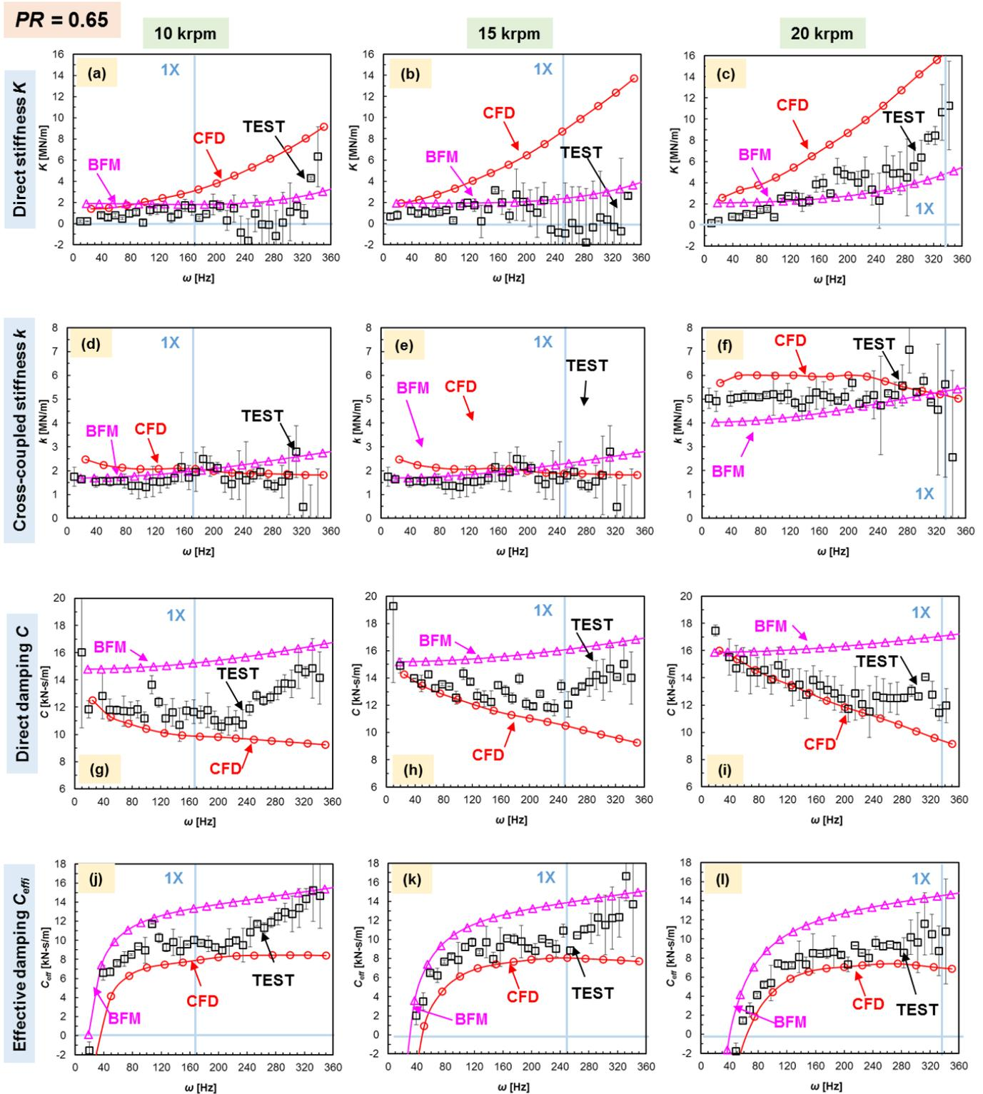
Figure 18 FPDS: test, CFD and BFM predicted force coefficients ( $K$ ,  $k$ ,  $C$ ,  $C_{eff}$ ) vs. frequency ( $\omega$ ) for  $P_{in} = 70$  bar,  $PR = 0.65$ . Shaft speeds: 10, 15 and 20 krpm ( $\frac{1}{2}\Omega D = 60$  to 120 m/s), zero inlet pre-swirl condition.
