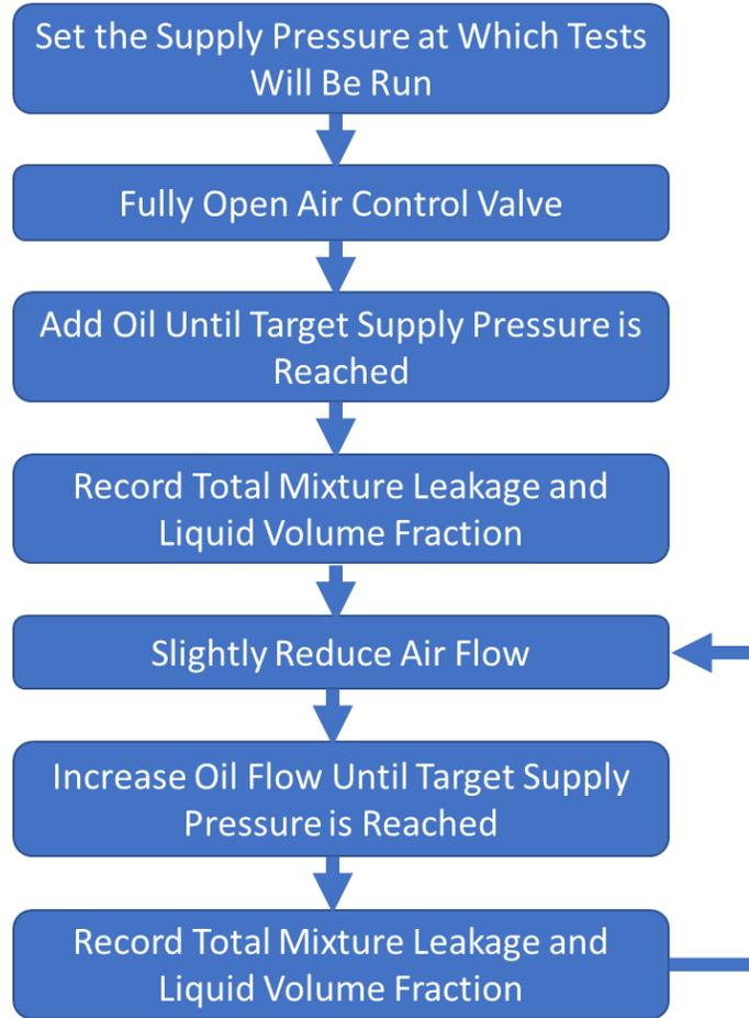
**Fig. 7. Experimental Procedure for Measurement of Seal Leakage at a Target Supply Pressure, LVF Range, and Rotor Speed.**
