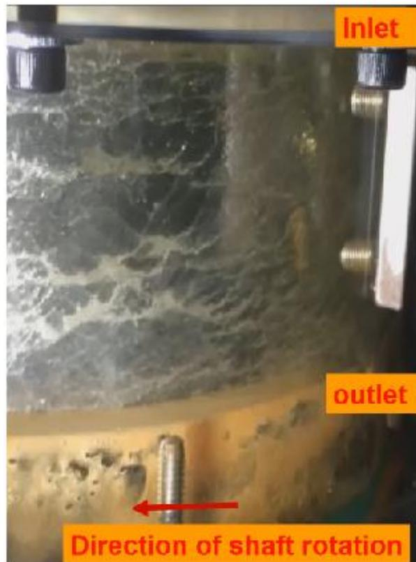
Figure 2 Flow visualization of wet seal operating with a gas and oil mixture. Inlet GVF = 0.9, journal speed = 1,800 rpm. Pictures taken with a stroboscope light at 30 Hz. Seal inlet pressure ( $P_s$ ) = 2.0 bar (a), discharge pressure ( $P_a$ ) = 1 bara. Picture reproduced from Ref. [11].
