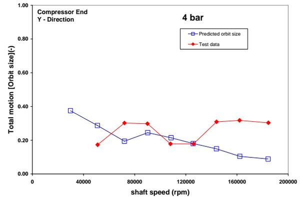
Fig. 4 Nonlinear prediction and test data of total shaft motion magnitude at compressor end versus rotor speed.
