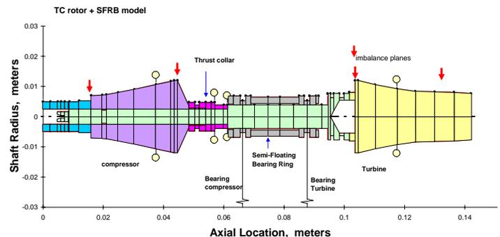
Fig. 1 Structural FE model of turbocharger rotor and semi-floating ring bearing
