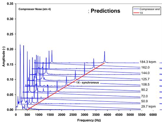
Fig. 3 Waterfall of predicted shaft displacements at compressor end. Conditions same as in Fig. 2
