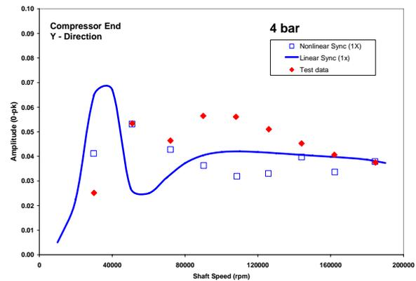
Fig. 5 Amplitude of shaft synchronous motion versus rotor speed. Test data, linear and nonlinear predictions
