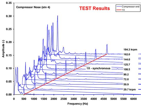
Fig. 2 Waterfall of measured shaft displacements at compressor end. Shaft speed range 30 to 184 krpm, 4 bar oil pressure and 93°C oil temperature
