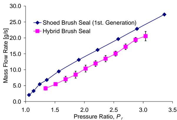
Figure 7. Test flow rates for 1<sup>st</sup> generation shoed-brush seal (SBS) and hybrid brush seal (HBS) versus supply to discharge pressure ratio under static conditions (no shaft rotation)
