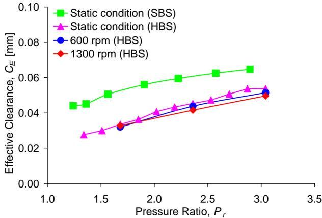
Figure 9. Calculated effective clearance for shoed-brush seal (SBS) and hybrid brush seal (HBS) versus supply pressure to discharge pressure ratio at static condition (no rotation) and selected shaft speeds (600 and 1,300 RPM)
