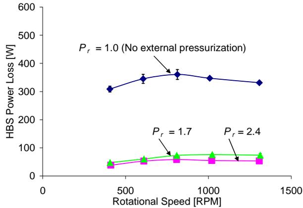
Figure 5. Test power loss for hybrid brush seal (HBS) versus rotational speed for increasing supply to discharge pressure ratios.
