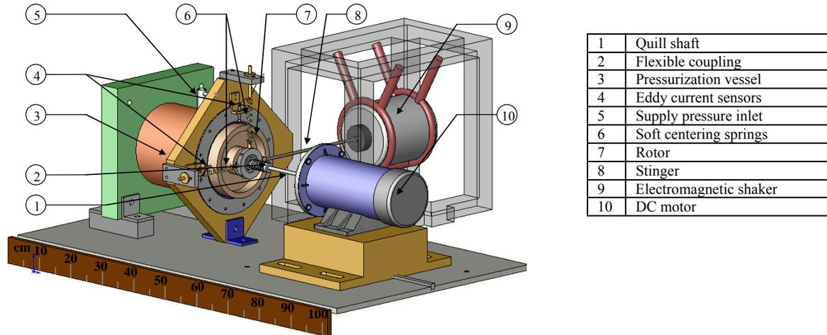
Figure 3. Rotordynamic test rig for a hybrid brush seal (HBS)
