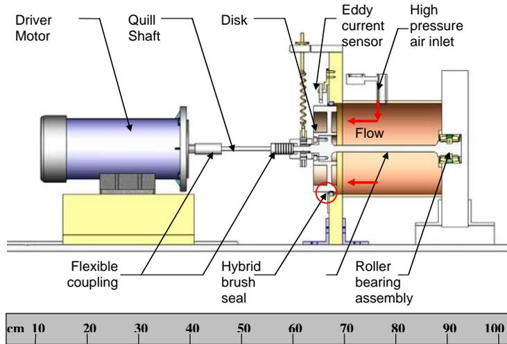
Figure 4. Cut view of hybrid brush seal rotordynamic test rig
