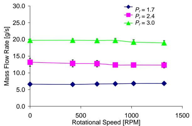
Figure 8. Test flow rate for hybrid brush seal (HBS) versus rotor speed for increasing supply to discharge pressure ratios
