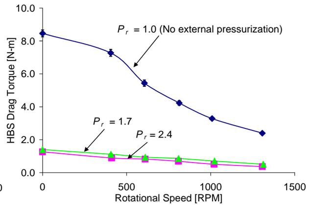
Figure 6. Drag torque for hybrid brush seal (HBS) versus rotational speed for increasing supply to discharge pressure ratios
