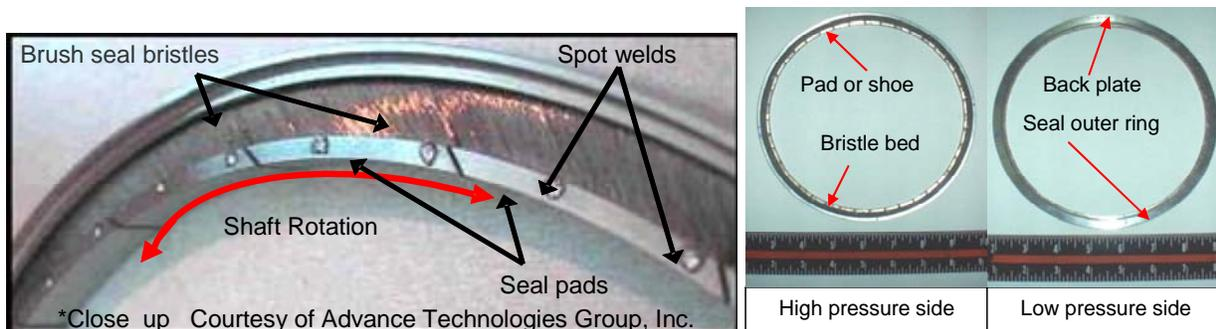
Figure 1. Close up view of shoed-brush seal (SBS) and back and front sides
