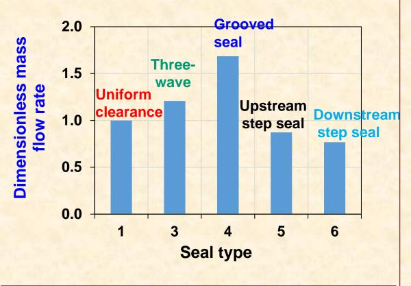
Three-wave seal leaks more than plain seal.
