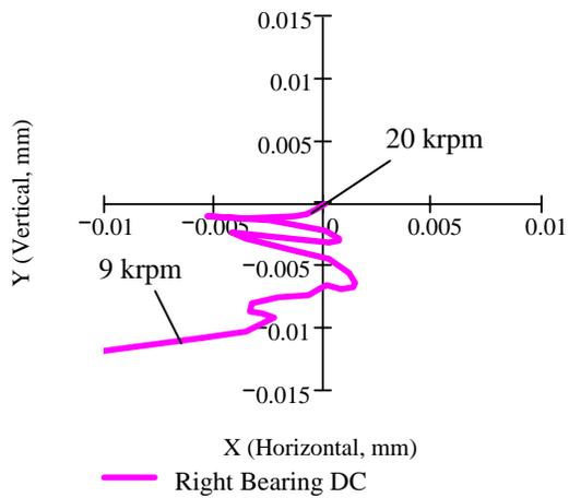
**Fig. 17 Shaft center static motions in vertical and horizontal planes for a test pressure 2.39 bar. Test bearing set #1**
