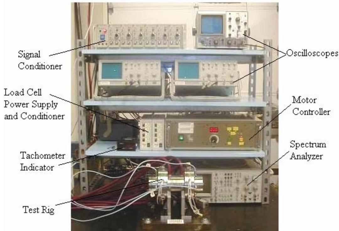
**Fig. 1 Gas bearing test rig and instrumentation**
