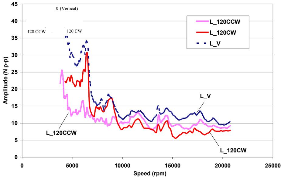
**Fig. 18 Overall components of bearing transmitted load peak-peak amplitudes at supply gas pressure of 5.15 bars. Test bearing set #1. L\_V-Left bearing vertical plane, L\_120CCW-Left bearing 120 counterclockwise from the vertical plane, L\_120CW- Left bearing 120 clockwise from the vertical plane.**
