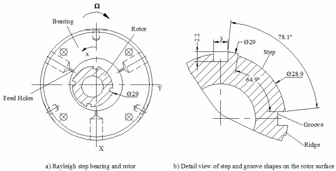
**Fig. 4 Schematic view of test Rayleigh step bearing and rotor; and a detail view of steps and grooves on the rotor surface (Units: mm)**
