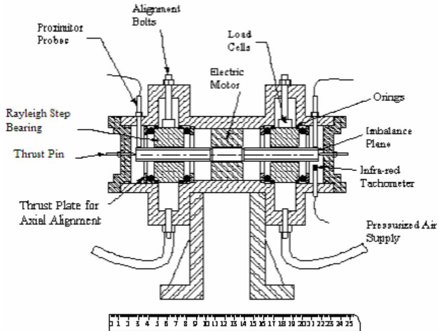
Fig. 2 Schematic cross section view of test rig (Unit: cm)
