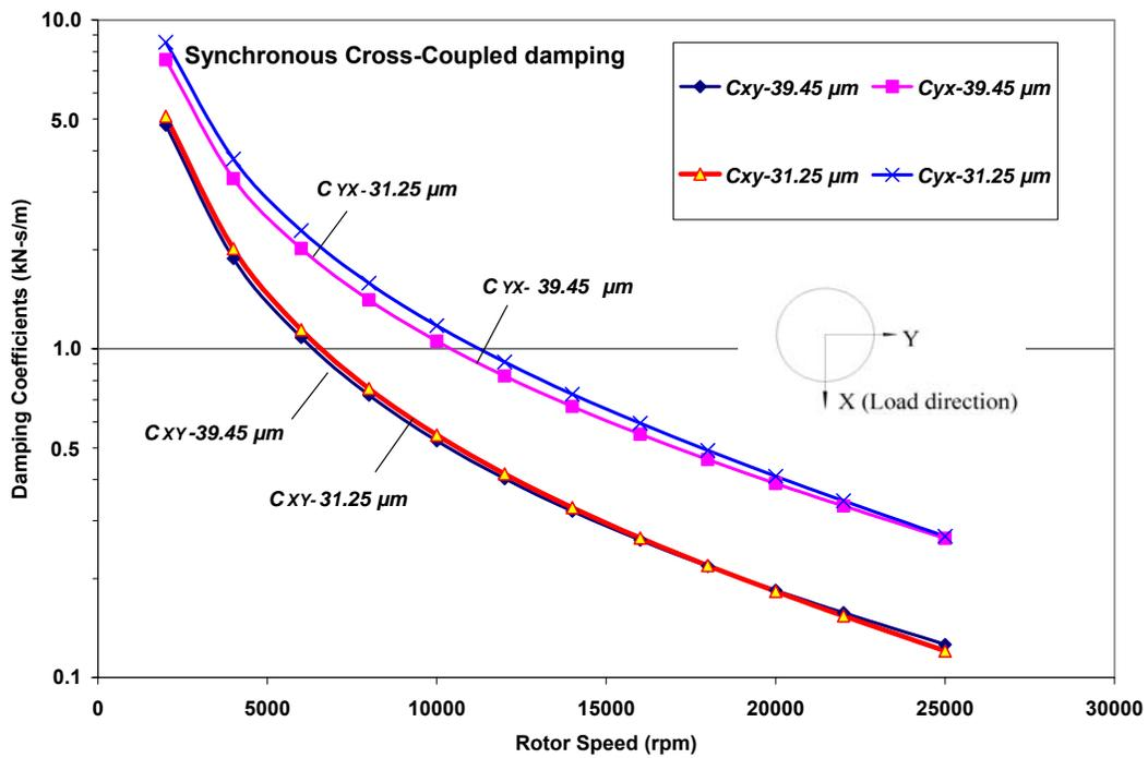
Fig. 38 Predicted synchronous direct and cross-coupled damping coefficients for bearings with radial clearances ( $C$ ) of 31.25  $\mu\text{m}$  and 39.45  $\mu\text{m}$
