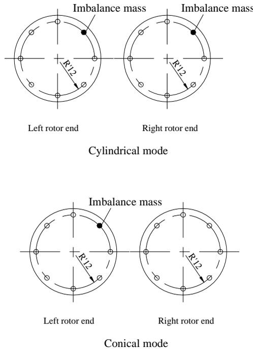
**Fig. 24 Imbalance mass locations at rotor ends for cylindrical and conical mode excitation**
