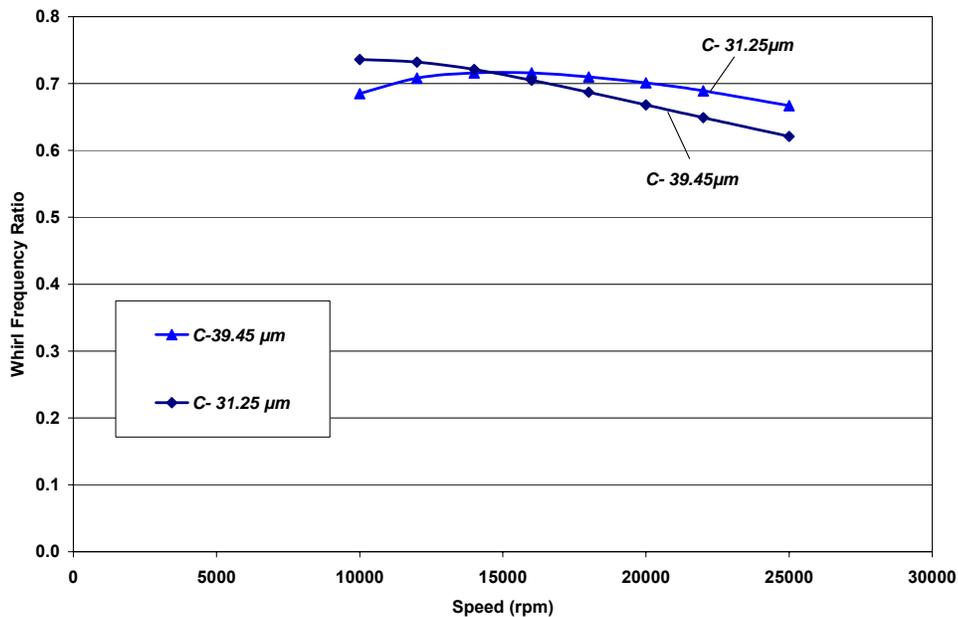
**Fig. 42 Predicted whirl frequency ratio (WFR) versus rotor speed for bearings with radial clearances (C) of 31.25 μm and 39.45 μm.**
