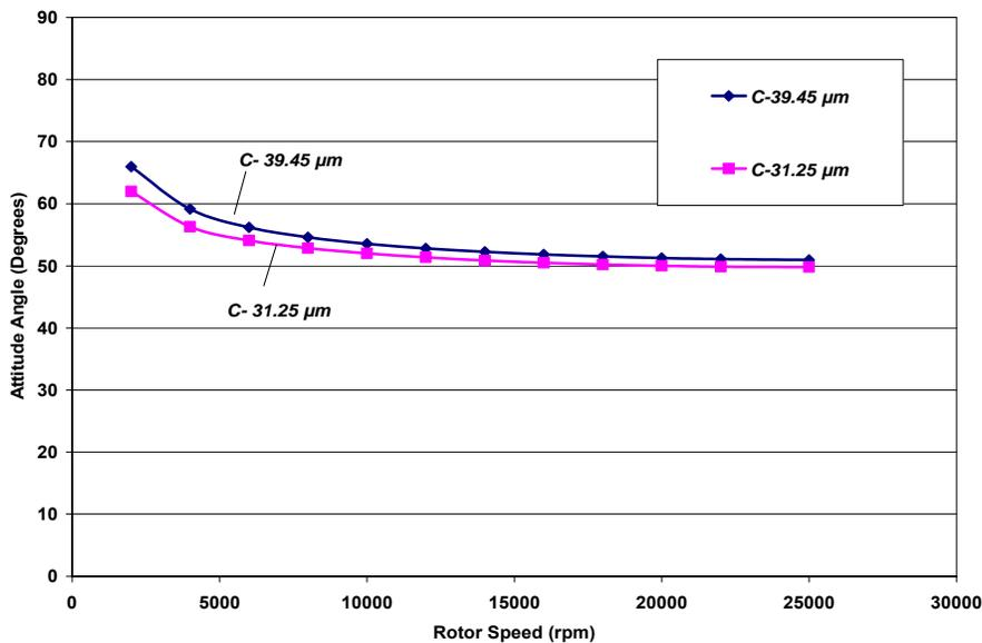
Fig. 34 Predicted attitude angles versus rotor speeds for bearings with radial clearances (C) of 31.25 µm and 39.45 µm
