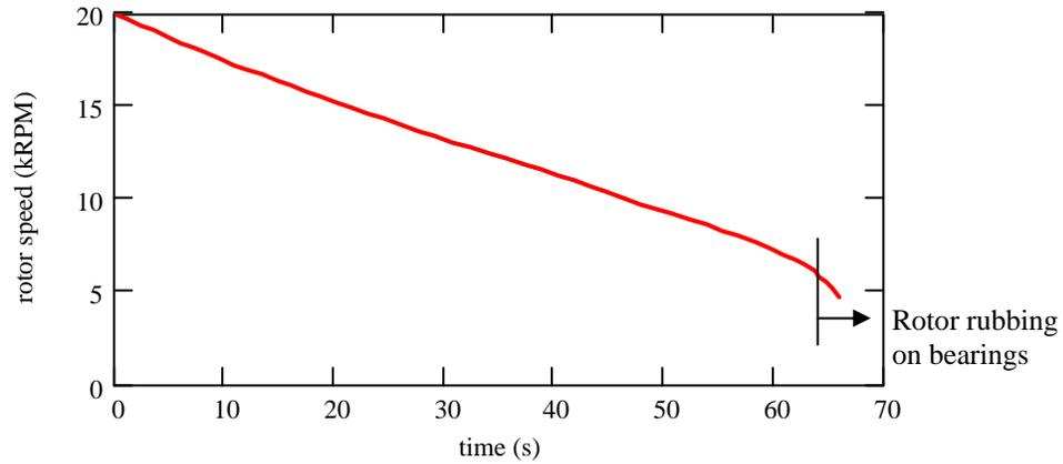
**Fig. 15 Typical rotor coastdown speed versus time for test bearing set #1 with supply gas pressure of 2.39 bar**
