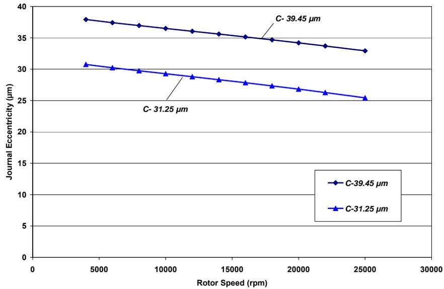
Fig. 33 Predicted journal eccentricities versus rotor speeds for bearings with radial clearances (C) of 39.45 µm and 31.25 µm
