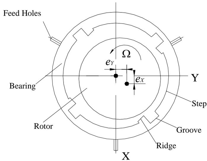
Fig. 32 Schematic view of geometry for rotor performance predictions with supported Rayleigh step bearings
