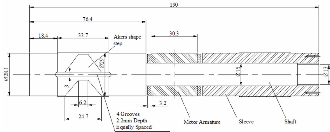
**Fig. 3 Geometry of test rotor with shaft, motor armature and bearing sleeves (Units: mm)**
