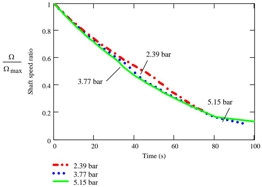
**Fig. A.3 Rotor coastdown speed ratio versus time for flexure pivot bearings with 20  $\mu\text{m}$  radial clearance at various feed gas pressures**
