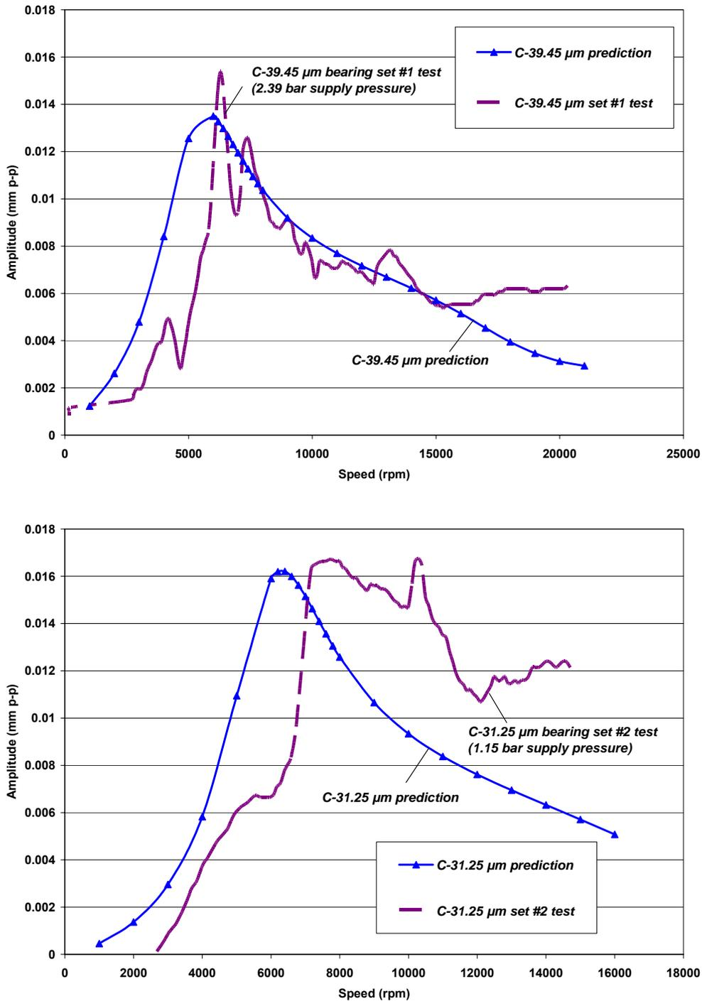
Fig. 44 Comparison of synchronous rotor displacement peak-peak amplitudes: predictions and test baseline at left bearing, horizontal plane. Test bearing sets with radial clearances ( $C$ ) of 39.45  $\mu\text{m}$  (top) and 31.25  $\mu\text{m}$  (bottom).
