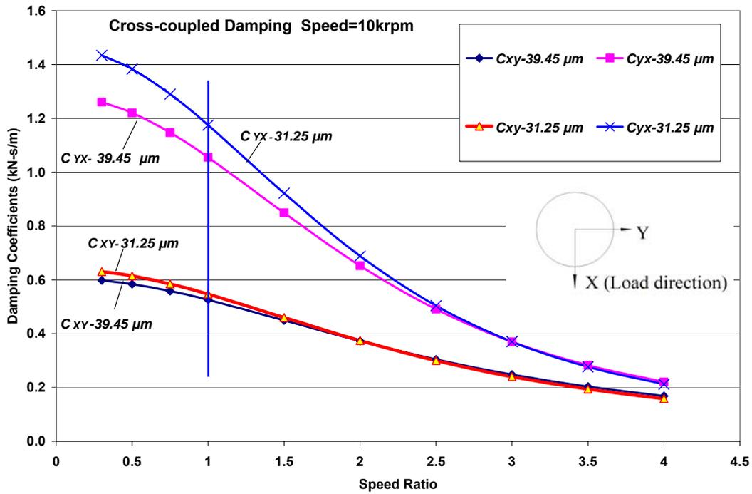
Fig. 41 Predicted effect of excitation frequency on bearing damping coefficients for rotor speed of 10 krpm. Bearings with radial clearances ( $C$ ) of 31.25  $\mu\text{m}$  and 39.45  $\mu\text{m}$
