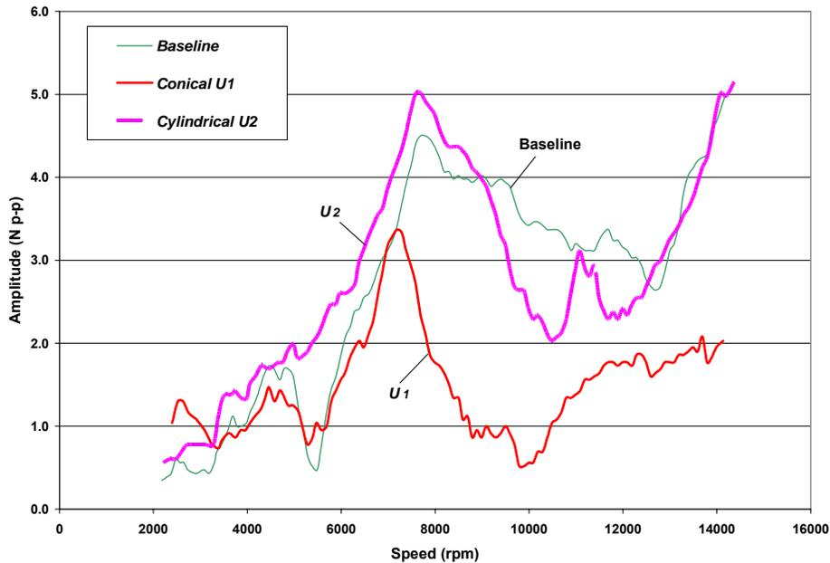
**Fig. 26 Synchronous bearing transmitted load peak-peak amplitudes for the rotor baseline and calibrated imbalance responses collected at the left bearing plane, 120° clockwise to the vertical direction. No external supply gas pressure. Test bearing set #2**
