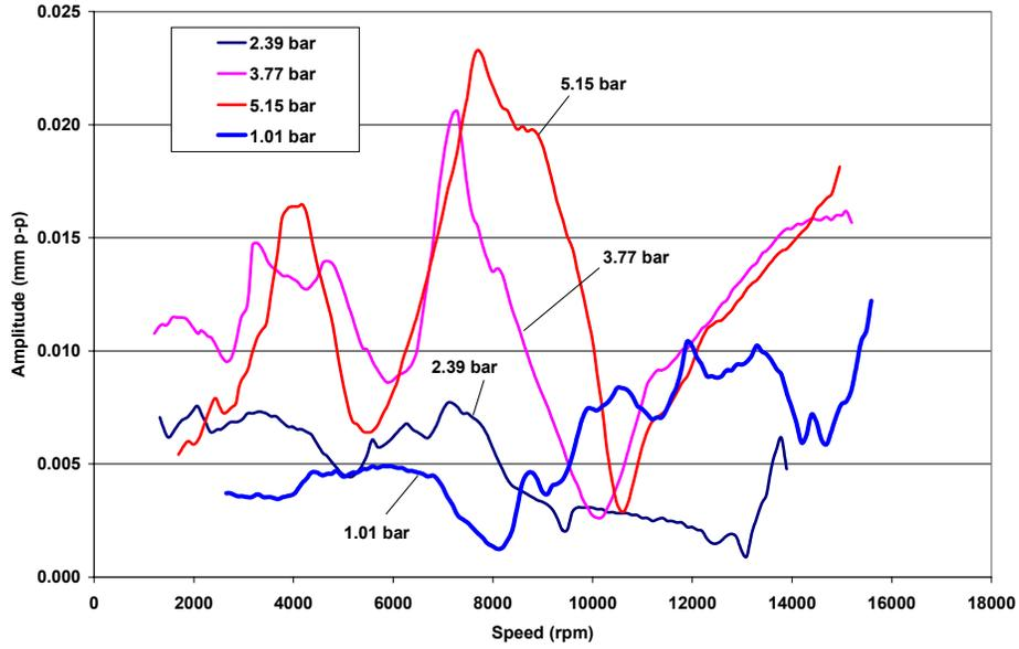
**Fig. 22 Synchronous rotor displacement peak-peak amplitudes for various supply pressures, recorded at left bearing, vertical plane (without slow roll compensation). Test bearing set #2**
