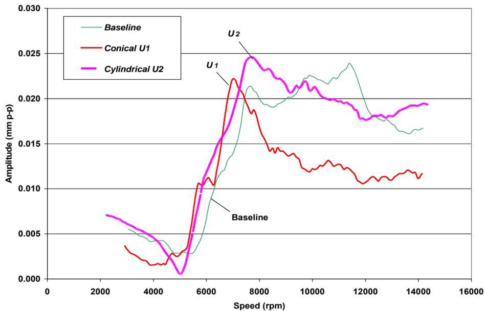
**Fig. 25 Synchronous displacement peak-peak amplitudes for the rotor baseline and calibrated imbalance response, recorded at the left bearing horizontal plane, without slow roll compensation. No external supply gas pressure. Test bearing set #2**
