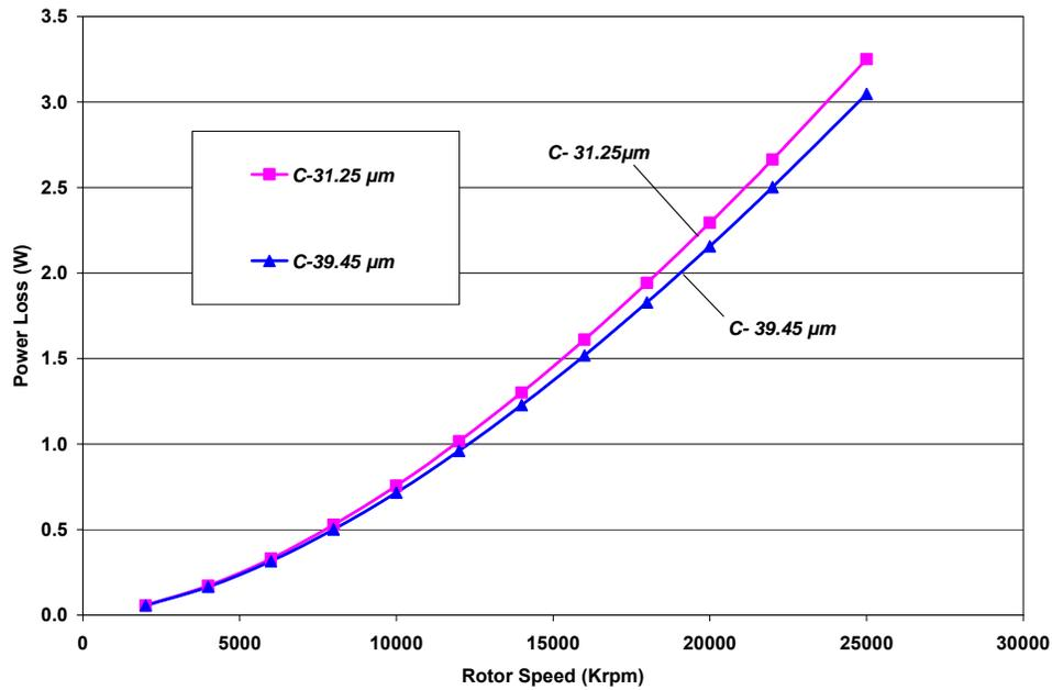
**Fig. 35 Predicted power loss for bearings with radial clearances (C) of 31.25 μm and 39.45 μm, respectively**
