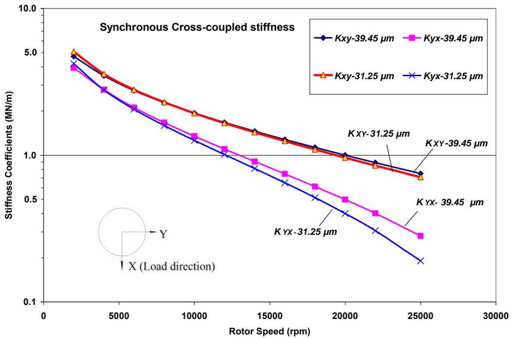
Fig. 37 Predicted synchronous direct and cross-coupled stiffness coefficients for bearings with radial clearances ( $C$ ) of  $31.25 \mu m$  and  $39.45 \mu m$
