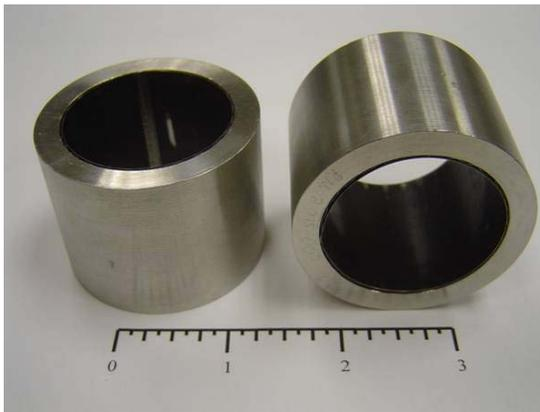
**Figure 2 Test bump type foil bearings**
