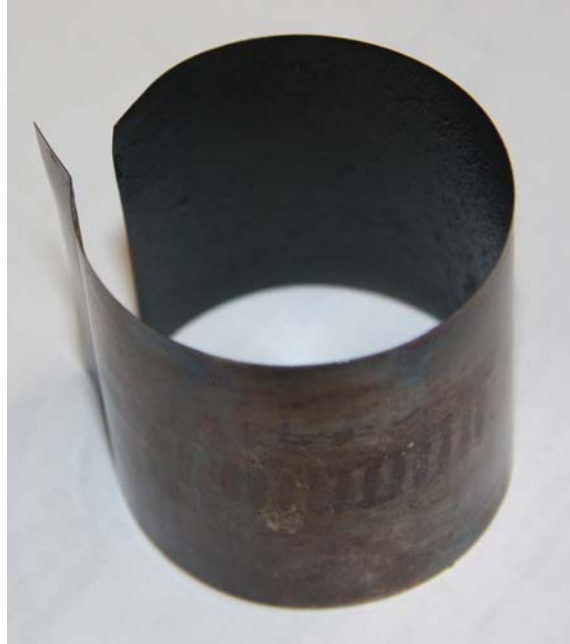
Fig. A.3 Top foil before assembly in a MMFB. The inner surface of the top foil coated with MoS 2
