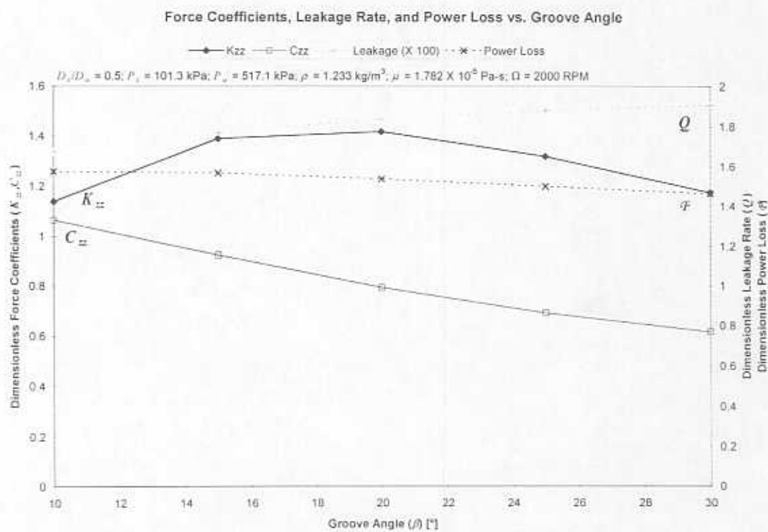
Figure 8. Variation of force coefficients, leakage rate, and power loss with groove angle ( \beta ).
