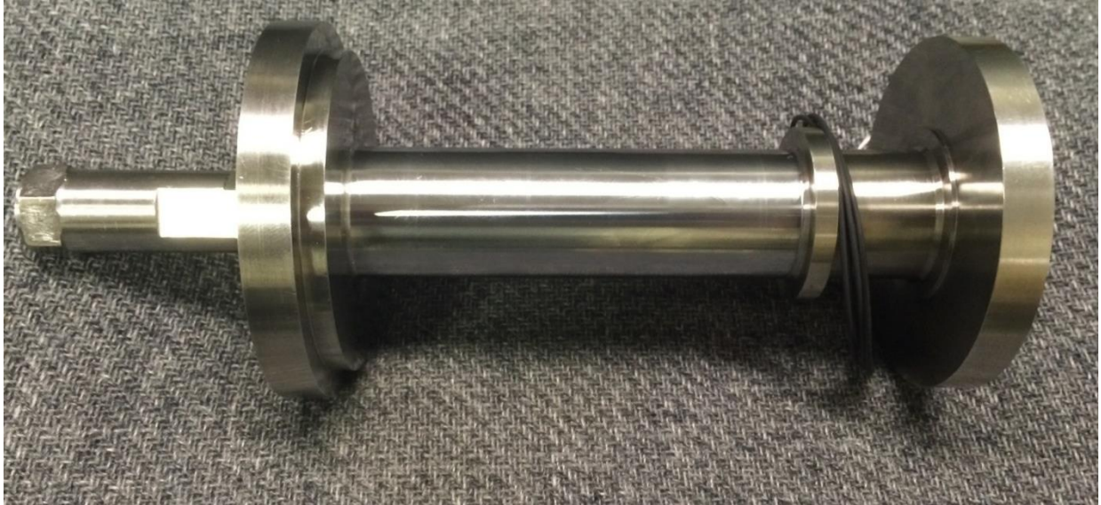
Figure 23. Photograph of rotor after being polished, pre-grinded, chrome-plated, post-grinded, and balanced (March 2014).
