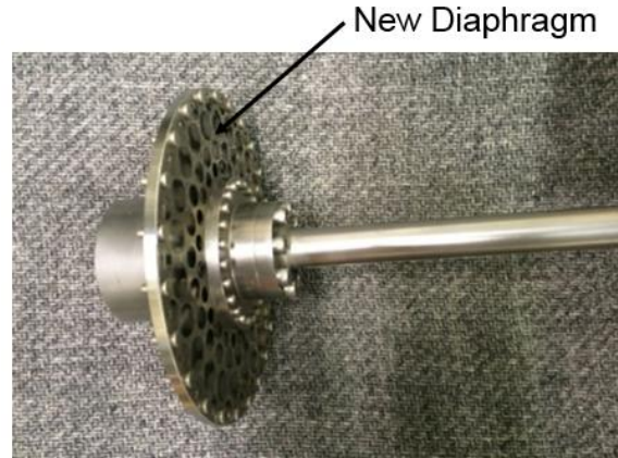
Figure 26. Photograph of flexible coupling after repair by Coupling Corporation of America.
