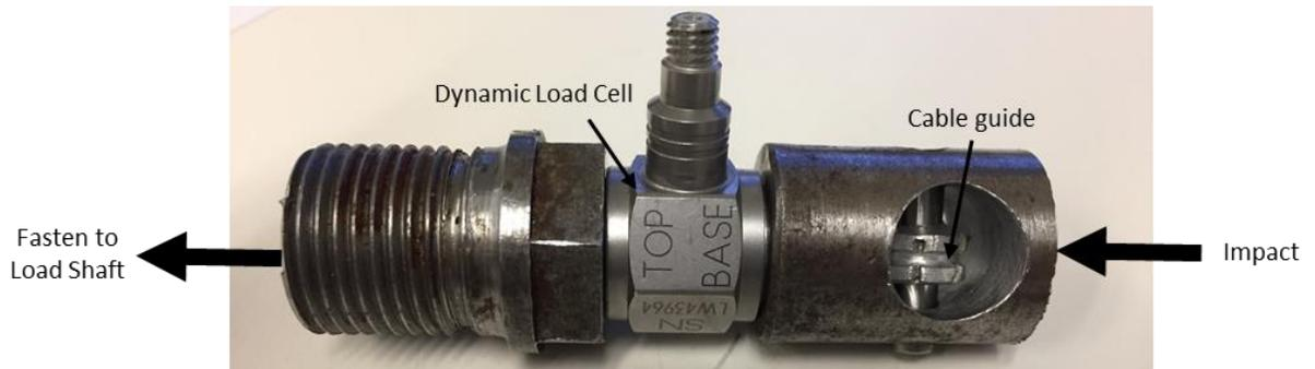
Figure 9: Loading Assembly for static and dynamic loading
