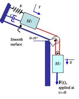
Static equilibrium position defines origin of coordinates X, Y describing the motion of blocks 2 and 1, respectively.
