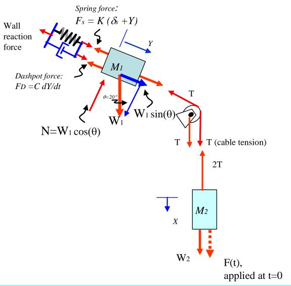
**(c)** for t>0, external force F(t) is applied to block 2.
