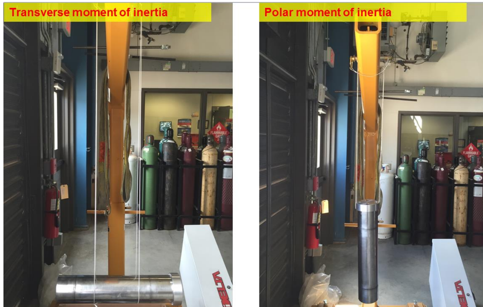
Fig. 3 Lab ad-hoc setups for recording period of natural motion (oscillation) of a suspended rotor.
