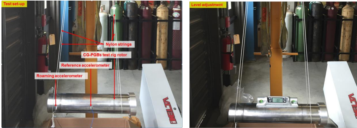
Fig. 4 Setup of rotor hanging from strings used for modal testing and identification of free-free modes.
