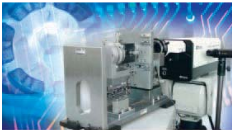
Noise investigation in hard disk spindle motors using scanning vibrometry
