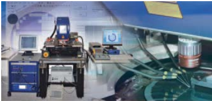
Semiautomatic, wafer-level measurements of MEMS dynamics
