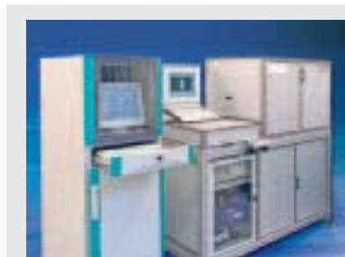
Semiautomatic test station based on a Compact Laser Vibrometer for quality control of medical devices
