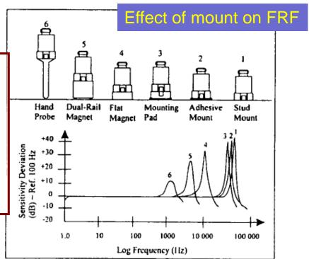
Figure 4. Assorted Mounting Configurations and Their Effects on High Frequency
