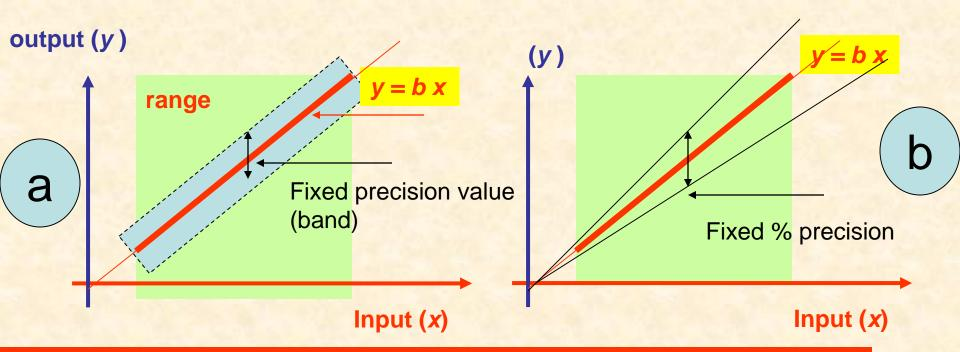
Sensor (a) is reliable for measurements at large *x* (upper end of range). Sensor (b) can be used for small *x* (lower end of range)
