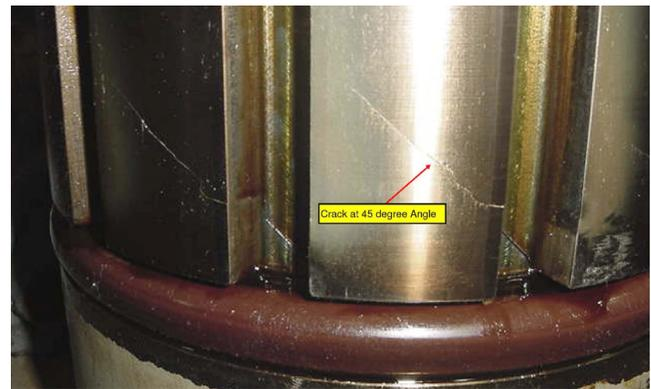
Figure 8. Failed Leaf-Spring Coupling.
