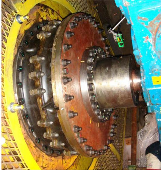
Figure 24. New Rubber-in-Shear Coupling.
