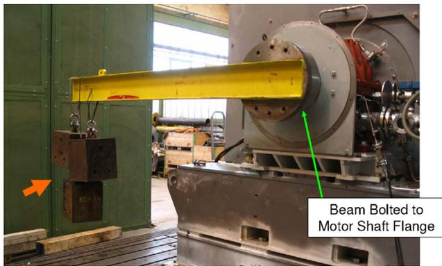
Figure 40. Weights Attached to Beam.
