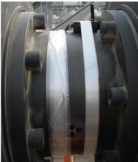
Figure 37. Strain Gage Telemetry System Installed on Coupling Spool Piece.
