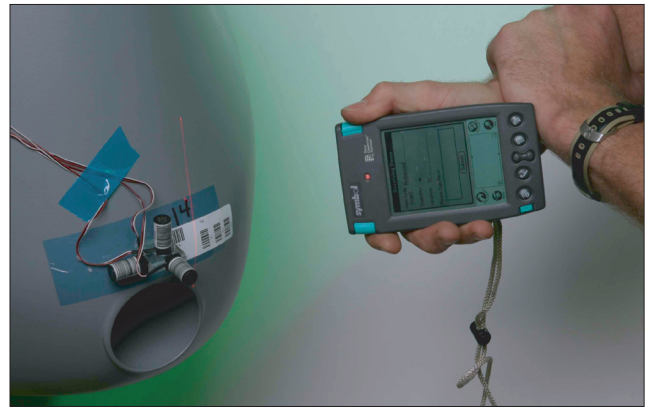
Figure 6. Using a Palm Pilot to scan the setup information reduces errors and improves efficiency.
