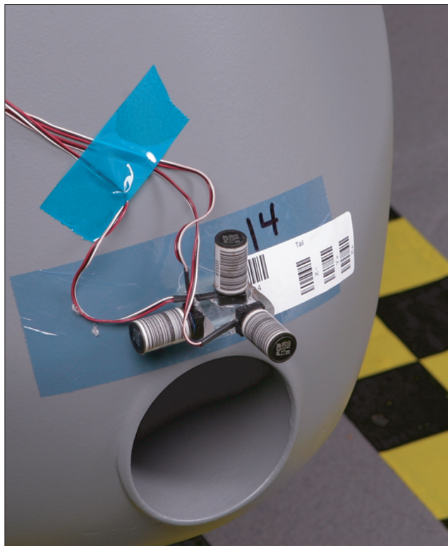
Figure 2. Typical accelerometer attachment using hot glue and a mounting block.
