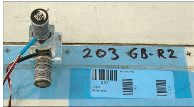
Figure 7. The use of bar codes, non-residue tape and hot glue enhance the accelerometer installation.
