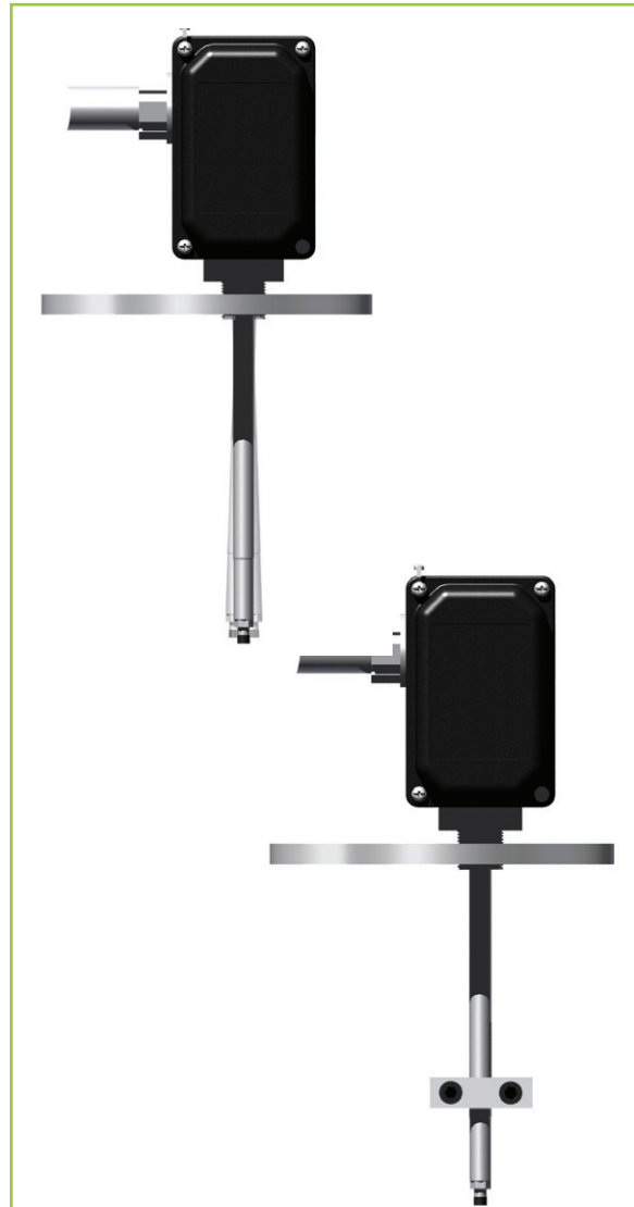
Figure 5. The probe on the top has a long unsupported length, resulting in mechanical resonance and erroneous readings as the probe is no longer stationary with respect to the shaft it observes. The probe on the bottom is identical, but has a mounting bracket to support and stiffen the probe "stinger." This ensures that the machine's vibration will not excite the probe mounting's resonance.
